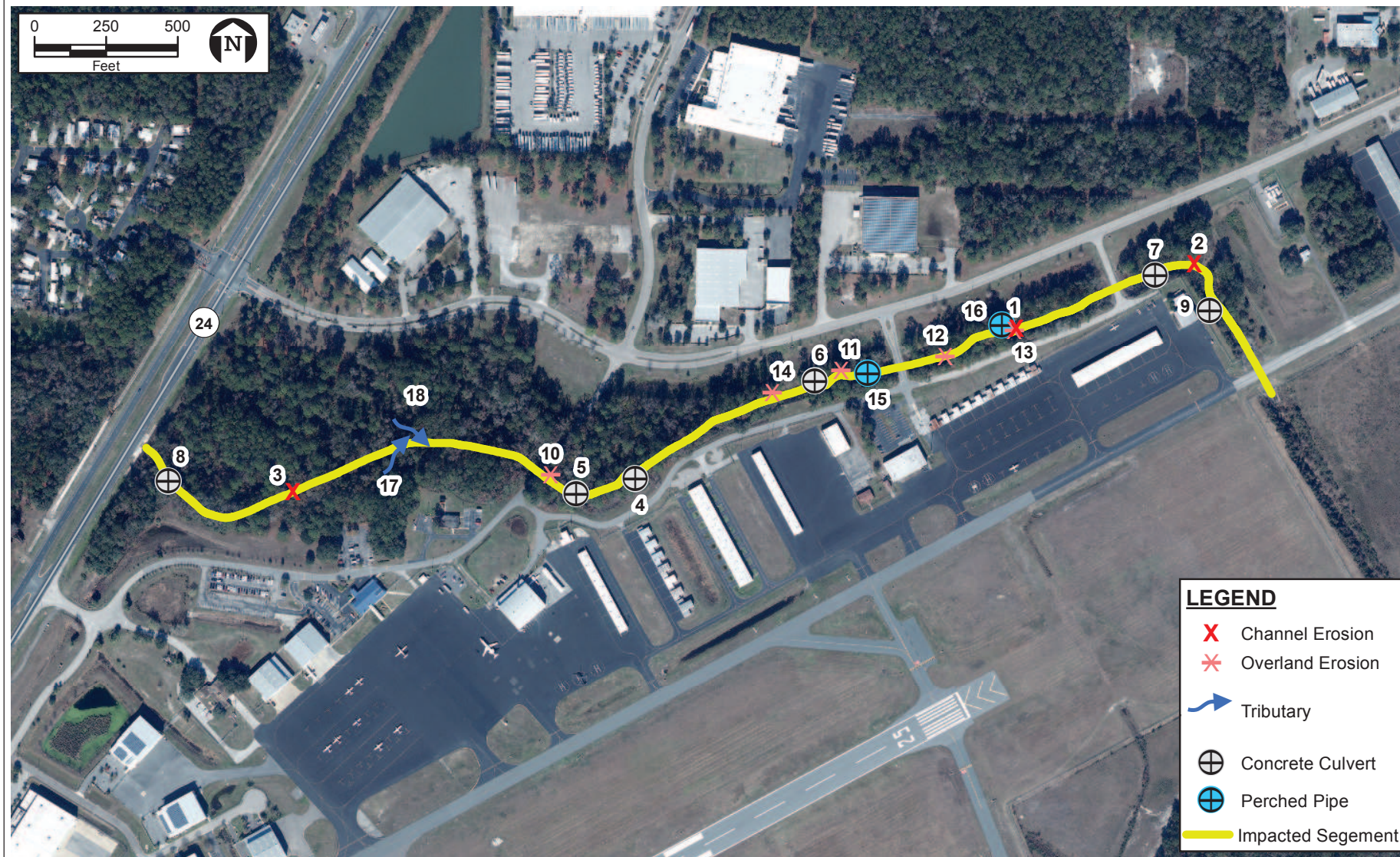
FIGURE 3-4. EROSION PROBLEM AREAS WITHIN LITTLE HATCHET CREEK IMPACTED SEGMENT
