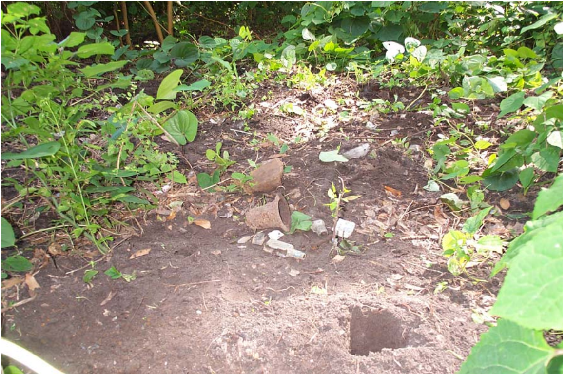
Image 1. Test boring with landfill debris present at the land surface.
