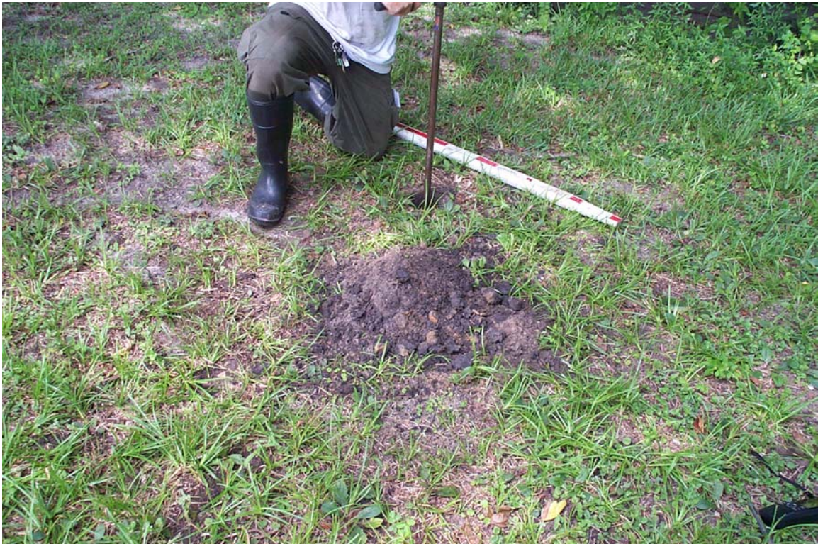
Image 23. Soil Boring 6, East side of Tumblin Creek, No Landfill Material Encountered
