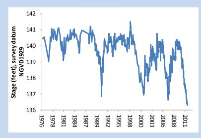
**Figure 4.** Graph of stage in Lake Alto(1976-2012) data collected by SRWMD.
