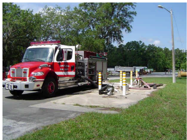
Pump testing a fire truck for Chiefland
