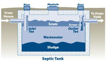
leaving the tank and traveling into the drainfield area. Screens are also recommended to keep solids from entering the drain field. The wastewater exits the septic tank and is discharged into the drain field for further treatment by the soil.
